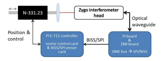
Fig. 1 Schematic representation of the experimental setup (image: PI)
