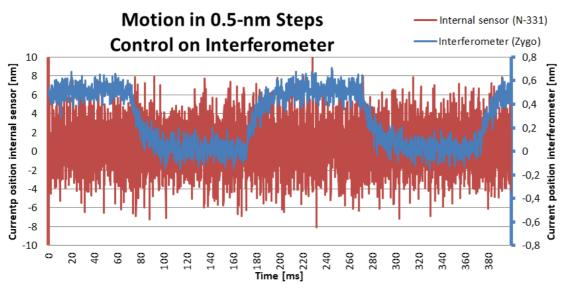
Fig. 2 Sensor signal at 0.5-nm steps - control on interferometer (image: PI)
