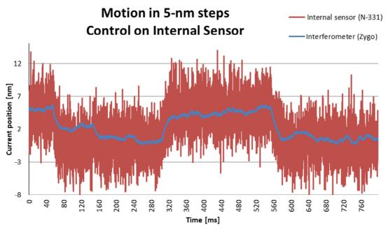
Fig. 1 Sensor signals at 5-nm steps - control on internal sensor (image: PI)
